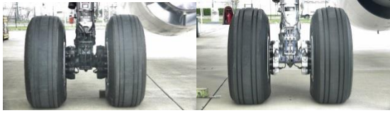
Figure 1. Captured images using PTZ camera a) Tires in bad condition b) Tires in good condition
